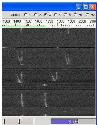
With the signal processing, one is able to decode signals buried in the noise of a typical SSB bandwidth. Signals down to ~ -30 dB below the noise, can be decoded given optimum conditions. The computer is looking at only a few Hz bandwidth, while our ears hear the noise over SSB bandwidth (2.4 kHz)
