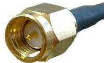
"Reverse polarity SMA" connectors sometimes used on WI-FI equipment has the gender of the connector reversed with its threaded body side having a centre pin instead of receptacle contact. This series led to the **SMB** (a very different design) and **MCX**, plus **SMC** often used hand-held radios for the antenna connector and looking similar to a reverse SMA.
