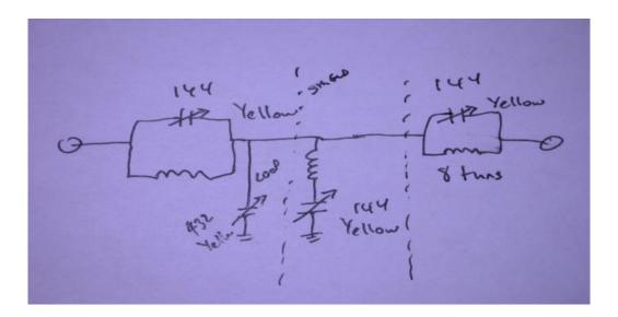
The 432MHz Band Pass tuned circuit consists of a loop of wire as shown below that is tuned with a Yellow "Phillips trimmer" that has a maximum capacitance of 10pF. The wire is approximately 20mm long and sits about 3mm above the ground plane. The 144MHz parallel and series tuned circuits are as above for the 144MHz filter. Placing some shields as depicted in the photographs below increases attenuation because of increased isolation from input to output.
