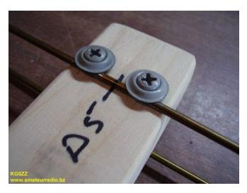
Add a plastic wire nut (twist on wire connector) to each end of all the elements.
