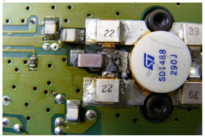
Burnt printed circuit board in the '9975 transmitter
