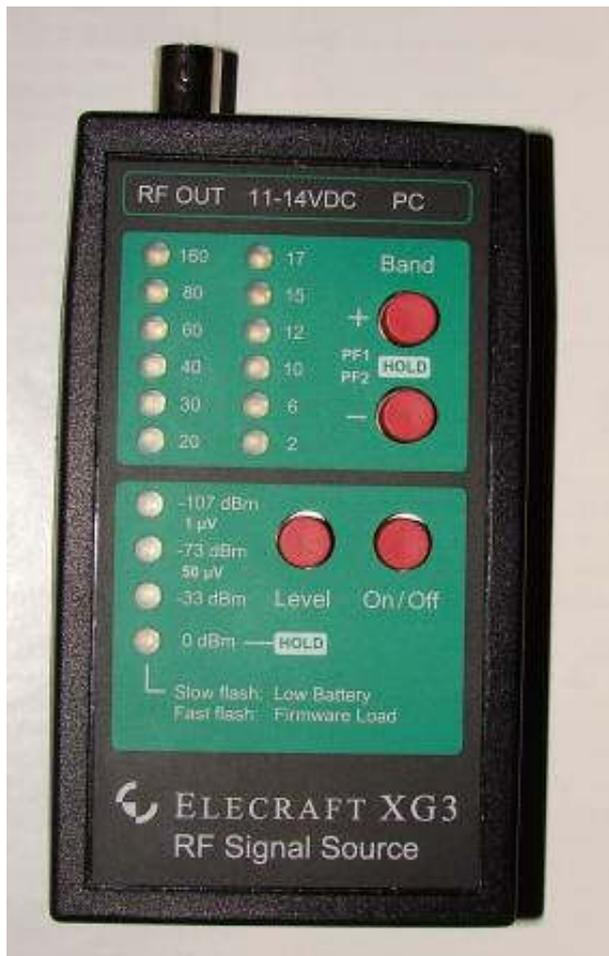
The scribe picked up a small Elecraft XG3 signal generator which uses a PLL IC and attenuation to give set levels (1  $\mu$ V, 50  $\mu$ V, 5mV and 223mV (0 dBm) for most amateur bands to 144 MHz. Runs on a PP3 9V battery and fits with my other portable kit.
