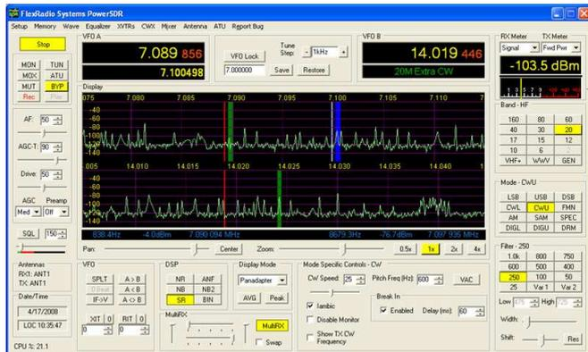
bandwidth, or looking for signal enhancement such as with antenna rotation, or via scatter off aircraft or other medium. The waterfall displays give an indication of signal level over time.
