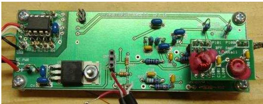
This is one of the Softrock RX kits built up as a single band unit. There is a switched Bandpass filter unit available, which allows reception across 1.8 thru 30 MHz. A new Programmable Oscillator IC allows tuning of the RX across
