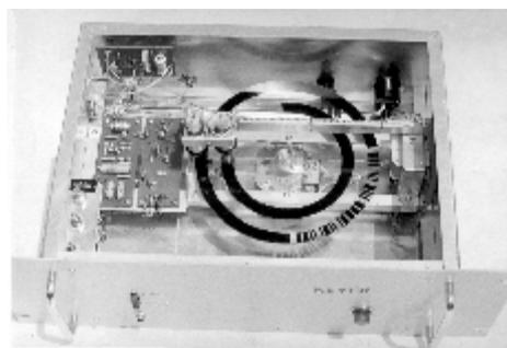
The keyer unit was self contained with its own internal power supply.
