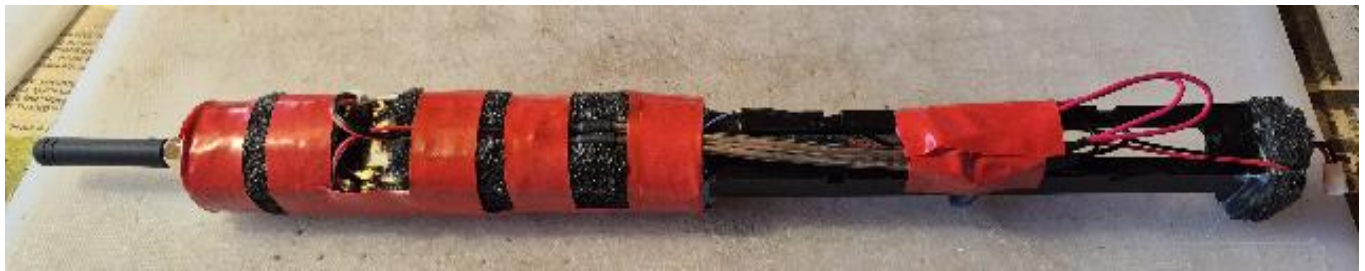
System assembly prior to installation within 40mm conduit housing. Stubby antenna on the left here is replaced by a 6dBi antenna in the final configuration (below).
