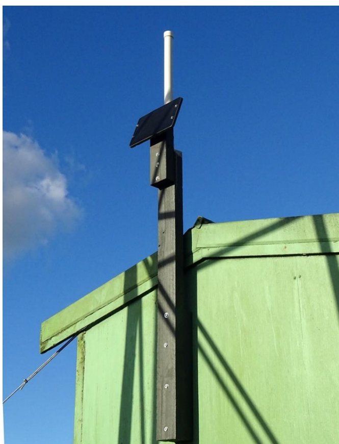
Meshtastic repeater , mounted above west wall of hut. This stand-alone solar powered repeater extends Waikato coverage into the Bay of Plenty.
