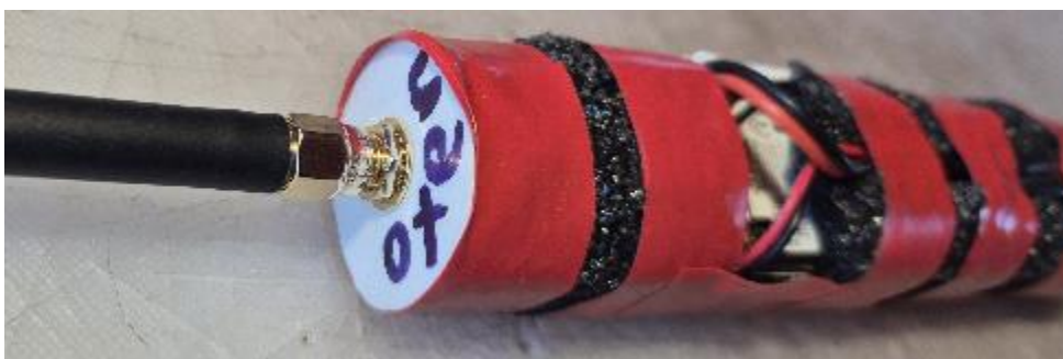
System assembly prior to installation within 40mm conduit housing. Stubby antenna on the left here is replaced by a 6dBi antenna in the final configuration (below).
