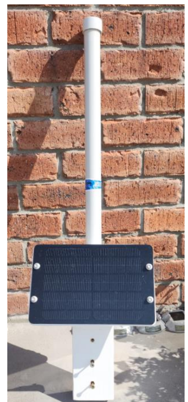
System assembly prior to installation within 40mm conduit housing. Stubby antenna on the left here is replaced by a 6dBi antenna in the final configuration (below).
